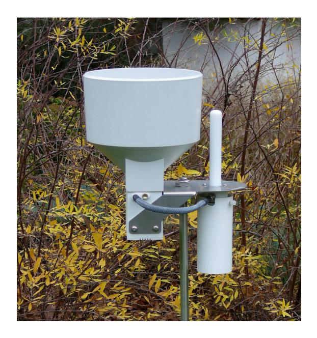
Precipitation and temperature sensor transmitting data via SigFox network to EMScloud Internet application.
